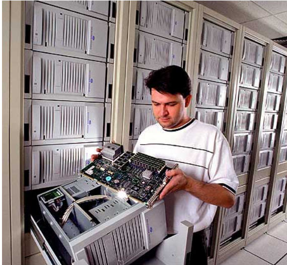
Ron Brightwell examines the motherboard of one of the Cplant's computers at Sandia National Laboratories. The board is from a 500A Digital personal workstation.
