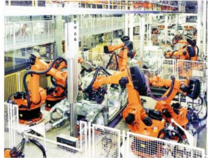
VW Zwickau, 2002: 650 robots welding car bodies for Golf and Passat 2
